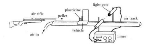
Describe how the apparatus is used to determine the speed of the vehicle.
